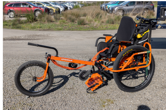
Pictured here, the AdvenChair is a human-powered, all-terrain wheelchair designed to enable individuals with mobility challenges to safely experience the serenity and grandeur of wild places with family and friends. Photo by Monique Trevett.
